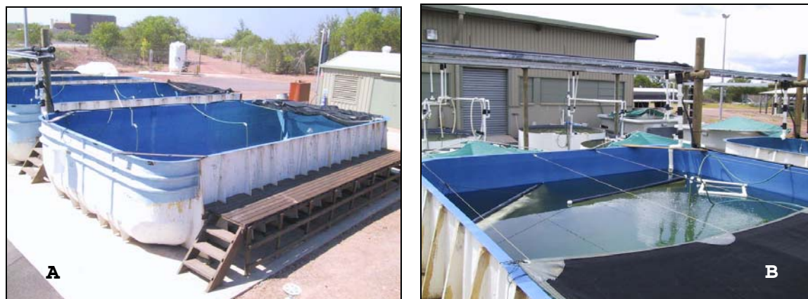
Figure 2. The two 40 m 3 tanks used for semi-intensive larval rearing of tropical marine finfish at the Darwin Aquaculture Centre. A. Tanks ready to be filled with chlorine-disinfected sea water. Aeration lines are suspended in the tanks; B. Tank under operation, half covered with 90% shade-cloth to control light levels. Feeder tanks containing extra zooplankton can be seen in the background.
